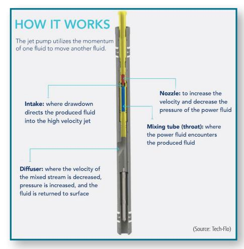
The jet pump itself has no moving parts, relying on a surface pump to move the fluid stream. With its small size and lack of moving parts, a jet pump is not affected by solids or gas locking and can be placed as deep as required by the well and formation. It rarely needs servicing and, when it does, it can easily be reversed out to replace the nozzle and mixing tube without the expense and downtime involved with a pulling unit.
